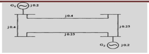
8. Find the bus impedance matrix for the system whose reactance diagram as shown below. All the impedances are in p.u. [L3] [CO1][10M]
