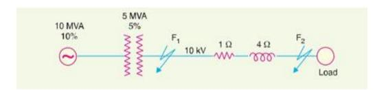
6. Consider the system shown in Fig below. The percentage reactance of each alternator is expressed on its own capacity determine the short circuit current that will flow into a dead  $3 - \emptyset$  short circuit at F.
